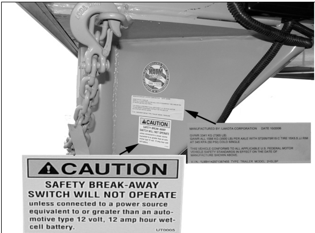
Figure 2-3 - Gooseneck Front Left Side Safety Warning And VIN Labels
