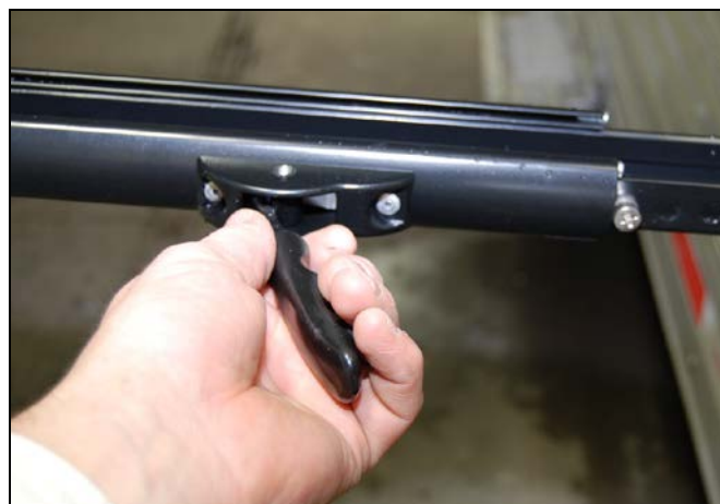
Figure 10-7 Awning arm adjustment latch
