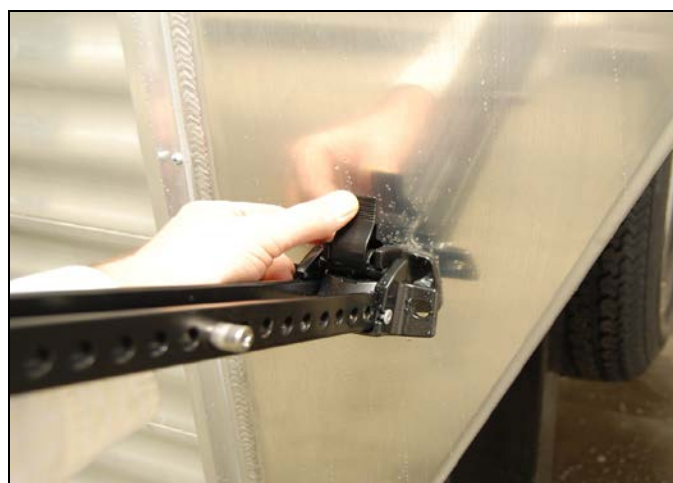
Figure 10-9 – Awning arm mounting latch
