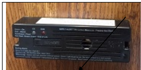
Figure 3-2 - LP Gas Detector
