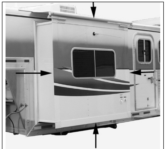
Figure 7-3 – Slide out Pinch Points
