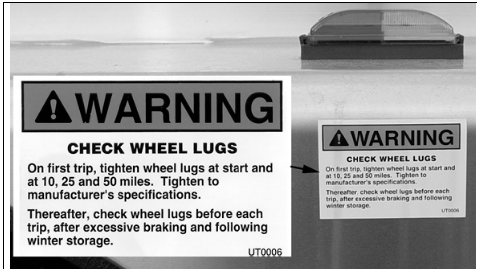
Figure 2-4 – All Trailers, Wheel Lug Safety Warning Label On Fenders
