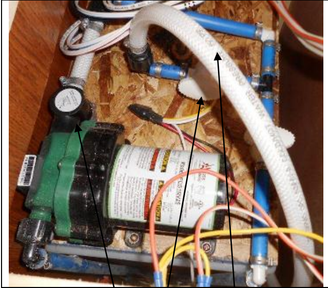
Figure 5-4 – Water Filter/Screen, Winterization line and valves
