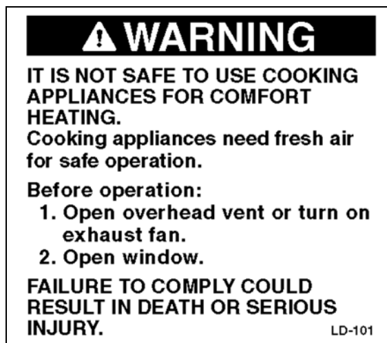
Figure 2-2 – Cook Top Safety Decal, Located On Inside And Outside Of Cook Top Lid
